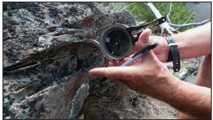
Figure 11. Use of tools in the field (e.g., Brunton compass) requires knowledge of how to use the instrument itself, and knowing where to make measurements, why this measurement should be made, and how it will be applied. Photo credit: Chuck Goodwin.
